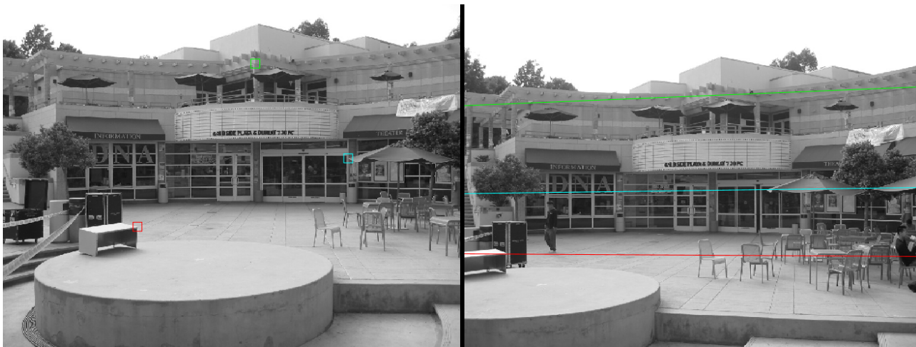
Figure 6: Three points \mathbf{x}_{1,2,3} in image_1 and the corresponding epipolar lines \ell'_{1,2,3} = \mathbf{F}_{LM}\mathbf{x}_i in image_2 . As it should, \ell'_i passes through \mathbf{x}'_i (the feature corresponding to \mathbf{x}_i ) in image_2 .
